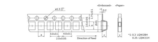
The dimension of the cavity of embossed tape is measured at the bottom side.
