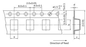
The dimension of the cavity of embossed tape is measured at the bottom side.
