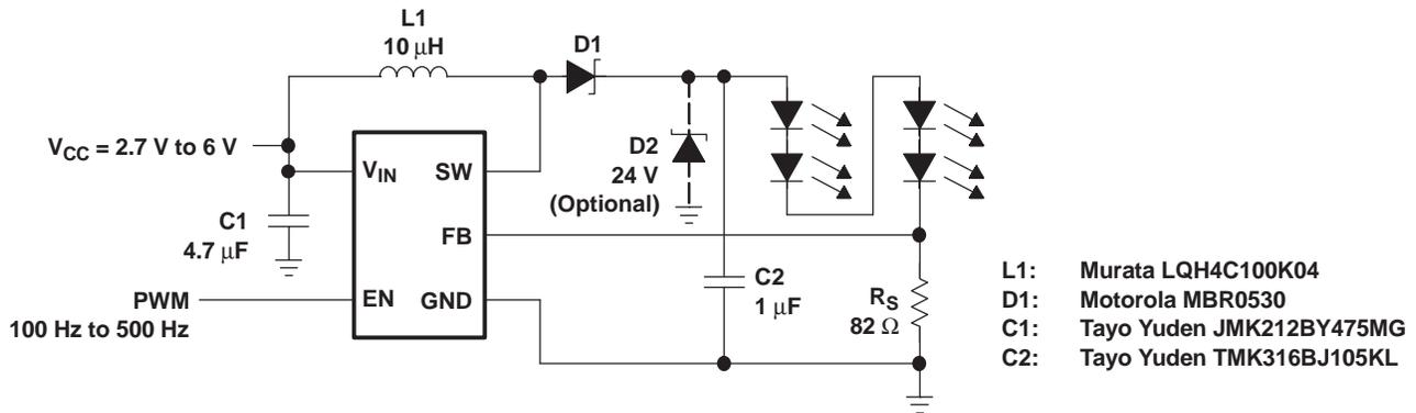
**Figure 22. White LED Supply With Adjustable Brightness Control**
