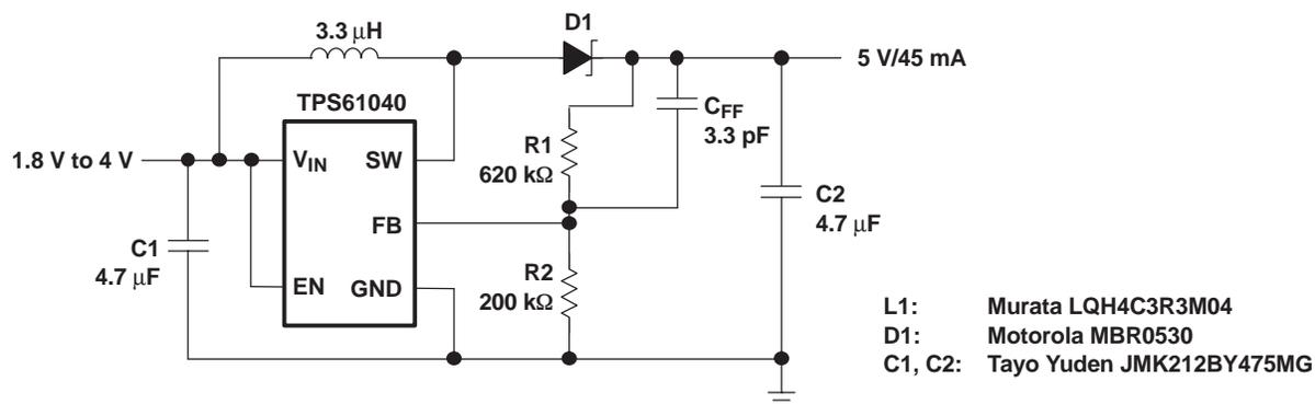
Figure 21. Dual Battery Cell to 5-V/50-mA Conversion
