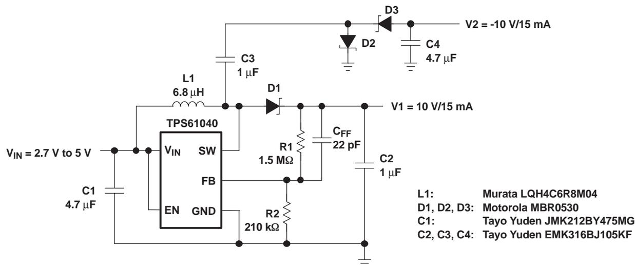
Figure 19. Positive and Negative Output LCD Bias Supply
