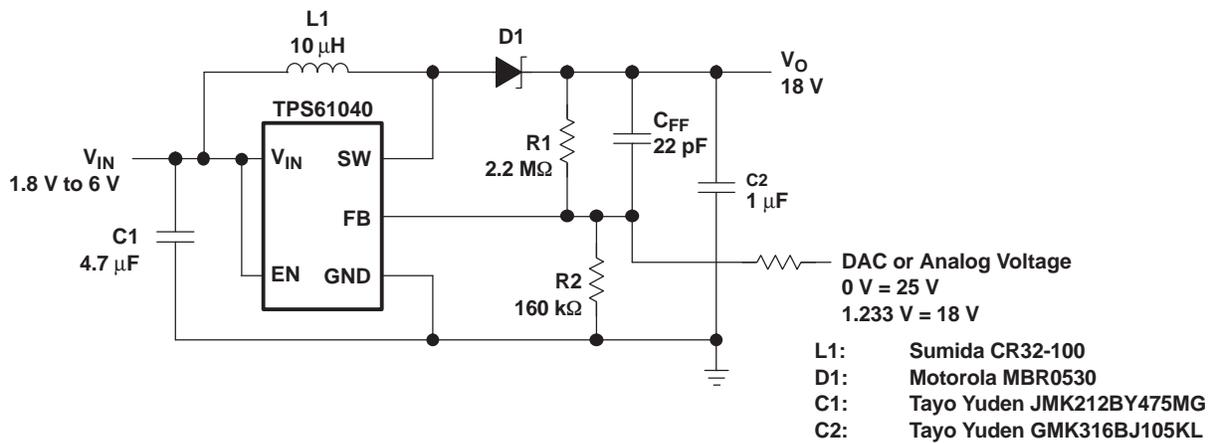
Figure 17. LCD Bias Supply With Adjustable Output Voltage
