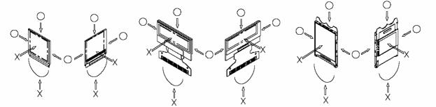
(7) Do not apply stress to the LSI chips and the surrounding molded sections.
