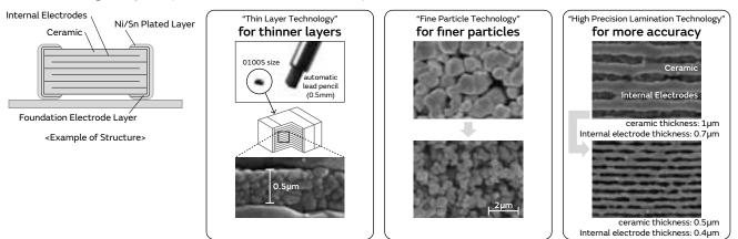
2 Sn plating is applied to the external electrodes; excellent solderability.
