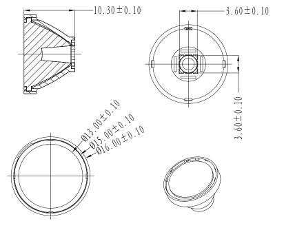
Notes: (1) All dimensions are in mm. (2) Drawing not to scale. (3) Collimator material is PMMA.
