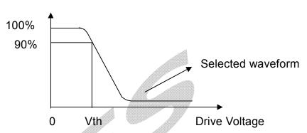
Vth: the voltage (Vop) which the brightness of segment indicates 10%,of saturated value on conditions.
