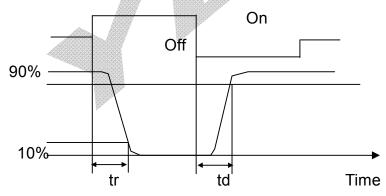
TR: THE TIME REQUIRED WHICH THE BRIGHTNESS OF SEGMENT BECOMES 90% FROM 0% WHEN WAVEFORM IS SWITCHED TO SELECTED ONE FROM NON-
