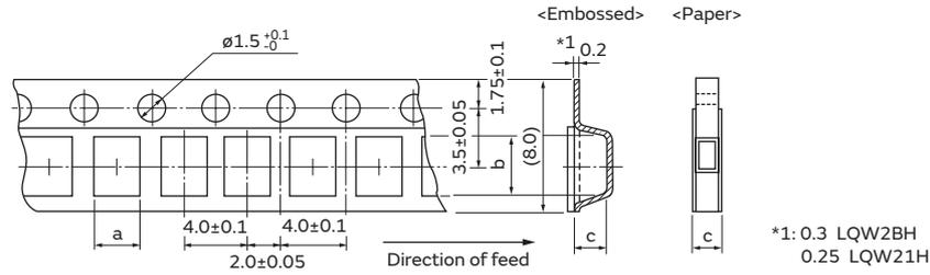
The dimension of the cavity of embossed tape is measured at the bottom side.
