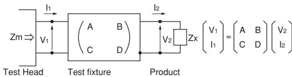
2. The impedance of chip Inductors (chip coils)  $Z_x$  and measured value  $Z_m$  can be described by input/output current/voltage.
